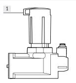
After setting the pressure, the rotary knob can be locked against unauthorised actuation.
