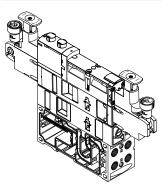
Additional function units can be added to each valve position between the base plate (manifold sub-base) and the valve. These functions are known as vertical stacking modules and enable special functions or control of an individual valve position. It is possible to link several valve sizes on one valve terminal.
