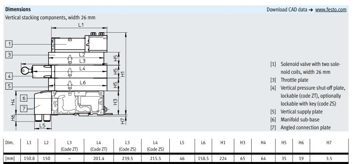
Vertical stacking components, width 26 mm
