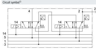
For the control block with safety function VOFA-B26-T52-... for the valve terminal, two 5/2-way solenoid valves of width 26 mm are pneumatically linked via two ducts, using an intermediate plate as vertical stacking element (output 2 is switched in parallel, output 4 is switched in series).
