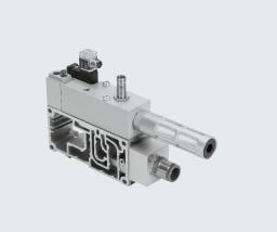
Once the working pressure in duct 1 reaches a previously set value, the soft-start valve switches to full operating pressure at duct 1 of the valve terminal.
