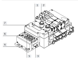
Electrical connection and display elements for VTSA-F-CB
