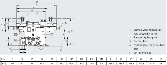
Vertical stacking components, width 18 mm, with the pressure regulator plate also suitable for valves with symmetrical design
