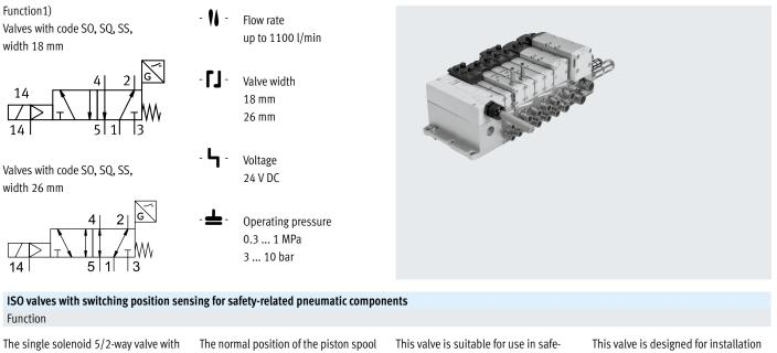
spring return in width 18 mm and 26 mm features valve diagnostics. It is available as a valve with plug-in or individual connection with pilot valves to ISO 15218 and square plug type C. The normal position of the piston spool is monitored by the inductive sensor. This valve is not a safety device in accordance with the Machinery Directive 2006/42/EC. When used in higher categories, the sensor signal from the valve must be evaluated by the control system.
