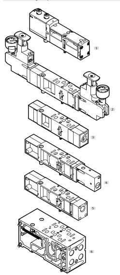
The following component sequence is recommended for valve positions with vertical stacking:
