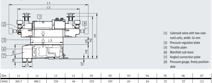
Vertical stacking components, width 26 mm, with the pressure regulator plate also suitable for valves with symmetrical design
