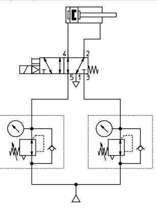
Circuit diagram 2: Pressure is regulated upstream of the valve
