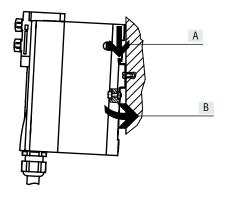
The valve terminal VTSA/VTSA-F/ VTSA-F-CB is hooked onto the DIN rail (see arrow A).
