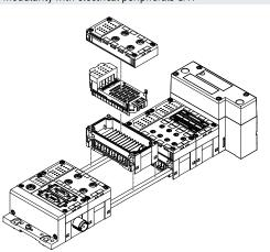
The metal CPX modules are mechanically connected using an angled fitting.
