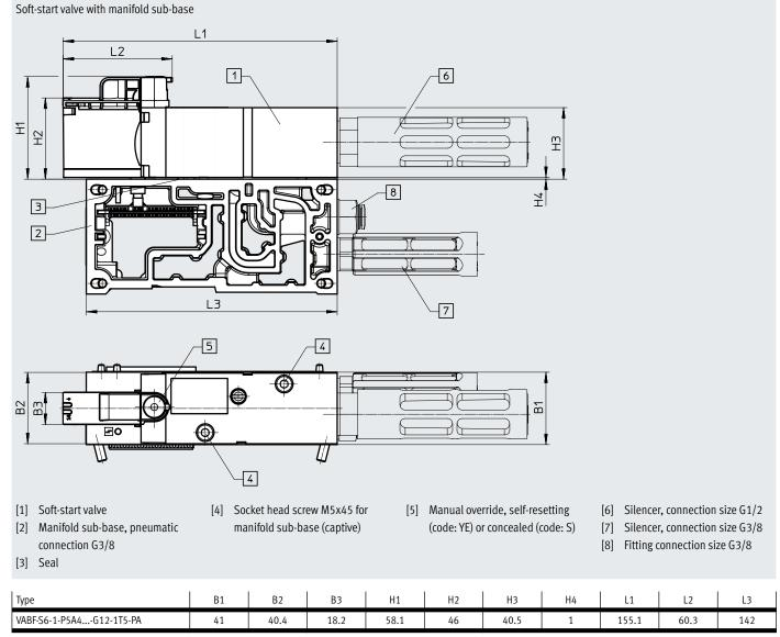
Seal <sup>1)</sup> between soft-start valve and manifold sub-base
