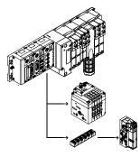
A controller integrated in the Festo valve terminal enables the construction of stand-alone control units with protection to IP65 without a control cabinet thanks to two different operating modes.
