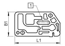
[1] With elongated hole, internal pilot air supply
