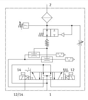
The vacuum generator is supplied internally via duct 1 of the manifold sub-base of the valve terminal. The pilot air is supplied internally via duct 12/14 of the manifold sub-base of the valve terminal.
