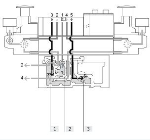
This pressure regulator regulates the pressure in ducts 2 and 4 after the pressure medium flows through the valve.
