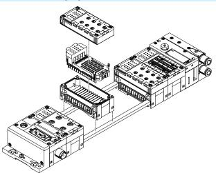
The CPX modules are mechanically connected to each other using tie rods. The entire unit can be assembled using two screws in the end plates.
