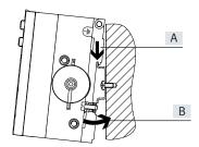
The valve terminal MPA-L is attached to the DIN rail (see arrow A).
