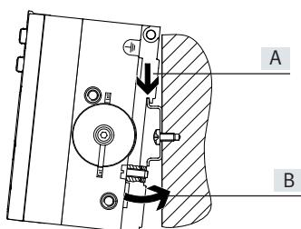
The valve terminal MPA-L is attached to the DIN rail (see arrow A). The valve terminal MPA-L is then swivelled onto the DIN rail and secured in place with the clamping element (see arrow B).
