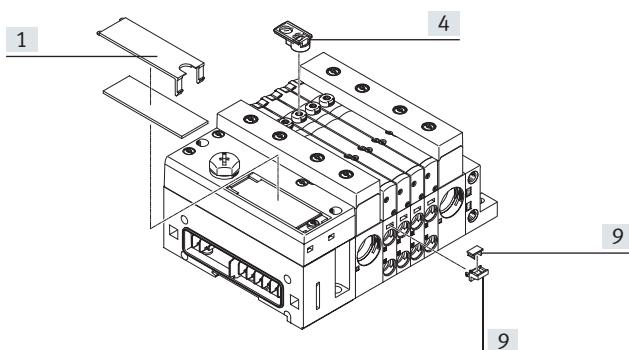
A label holder VMPAL-ST-AP-10 (part no. 561109) with identification labels (part no. 18576, IBS-6x10) can be mounted on each sub-base for labelling the valves.
