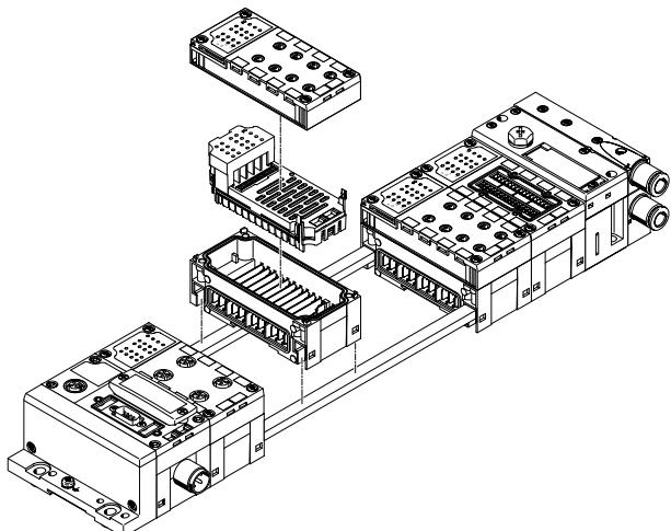
The CPX modules are mechanically connected to each other using tie rods. The entire unit can be assembled using two screws in the end plates.
