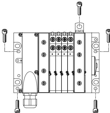
The valve terminal MPA-L is screwed onto the mounting surface using four M4 or M6 screws. The mounting holes are on the multi-pin plug connection and on the right end plate. Optional mounting brackets are also available.
