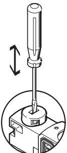
The MO is actuated by pushing it with a pointed object or screwdriver and reset by spring force (detenting position prevented due to cover cap).
