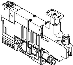
Additional functional units can be added to each valve position between the base plate and the valve.
