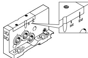
If the supply pressure (at the right end plate) is less than 0.3 MPa or greater than 0.8 MPa, then the valve terminal MPA-L must be operated with an external pilot air supply. The pilot air is then supplied via port 12/14 on the right
