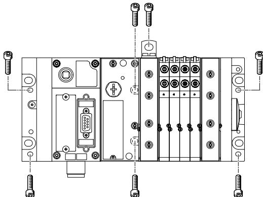
The valve terminal MPA-L is screwed onto the mounting surface using four M4 and two M6 screws or using six M6 screws. The mounting holes are on the left and right end plates and in the pneumatic interface. Optional mounting brackets are also available.
