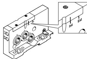
Internal pilot air supply can be selected if the supply pressure for the terminal is between 0.3 and 0.8 MPa.
