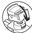
Clip the covering onto the pilot valve.
