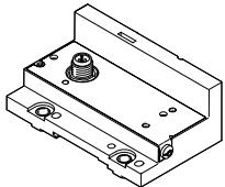
The electrical connection from the valves to a higher-order controller is in the left end plate of the MPA-L.
