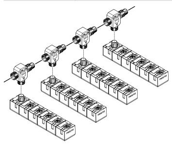
For a pure M12 installation, as an alternative to the looped-through AS-i bus, it is also possible to select an installation with spurs.
