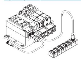
The compact I/O modules can be used to supplement the valve terminals VTSA/VTSA-F. The following are available:
