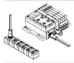
If an input module is at the end of a string, the flat cable can also be routed using a specially sealed fitting.
