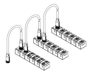
On this module, the supply of inputs is exclusively from the "yellow" AS-Interface cable, and the supply of outputs exclusively from the "black" AS-Interface cable. Power is supplied either completely via an M12 installation or via suitable converters.
