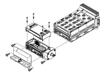
The mechanical connection between the CPX-AP-A modules is created using angled fittings.
