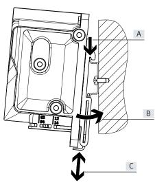
The valve terminal VTUX is attached to the DIN rail (see arrow A).
