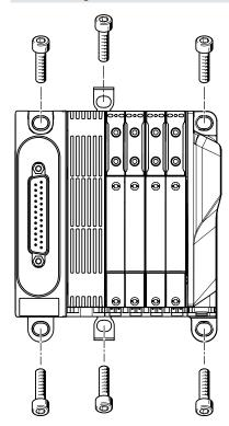
The valve terminal VTUX is screwed onto the mounting surface using four M4 or M6 screws. The mounting holes are on the multi-pin plug connection and on the right end plate.
