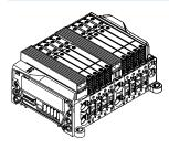
CPX-AP-A is a flexible, central, compact and lightweight remote I/O system with a high degree of protection to IP65/IP67.
