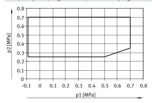
For 5/2-way valve, single solenoid, pneumatic spring return
