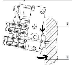
The DIN rail mounting VAME-T-M5 consists of two mounting clips. These are screwed onto the manifold rail on the left and right (M5 screws). The lower through-holes on the manifold rail are used for this.
