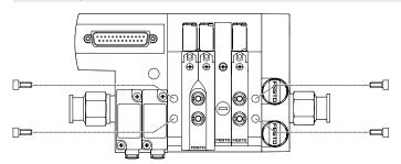
Sturdy terminal mounting thanks to four through-holes for wall mounting (M5 screws).
