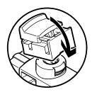
Turn MO to clip it onto the pilot valve. The MO cap can then be operated (detenting) without tools.
