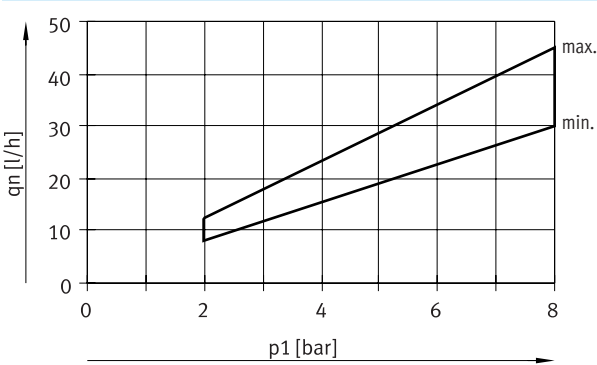
Internal air consumption qn as a function of operating pressure p1
