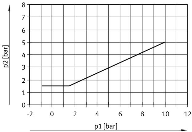
**Size 25 – Pilot pressure  $p_2$  as a function of working pressure  $p_1$**
