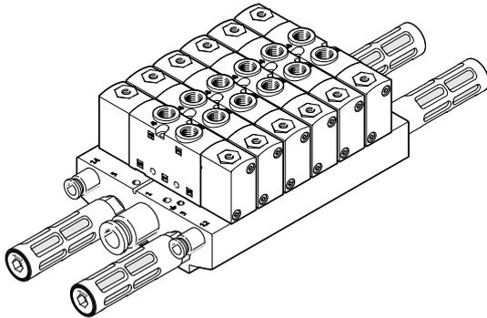
In-line valves are designed to be used without pneumatic links. All pneumatic connections are on the valve and can be equipped with fittings/tubing. By using a special seal set, the in-line valves can also be mounted on a manifold rail (pneumatic links) as semi in-line valves.
