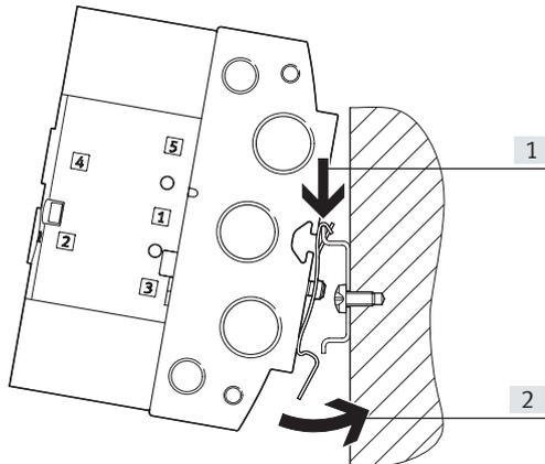
The DIN rail mounting VAME-T-M... consists of two mounting clips. These are screwed onto the manifold block on the left and right.
