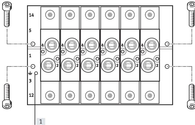
Sturdy wall mounting of the manifold block using four through-holes.
