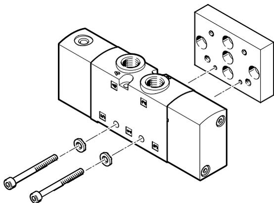
For mounting individual valves on a flat surface, e.g. aluminium profile systems.
