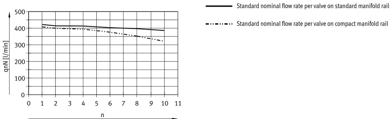
For 5/2-way valves, flow direction 1 → 4
