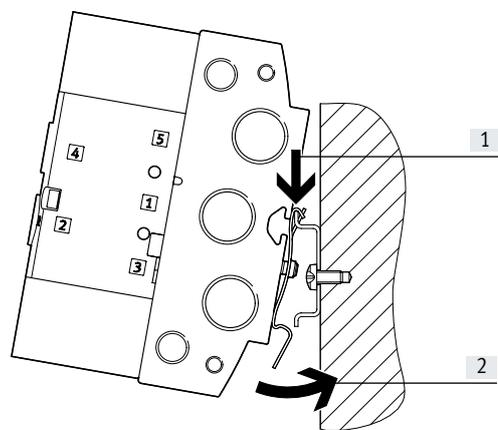
The H-rail mounting VAME-T-M... consists of two mounting clips. These are screwed to the manifold block on the left and right.
