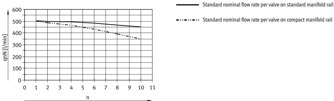
For 5/2-way valves, flow direction 1 → 2
