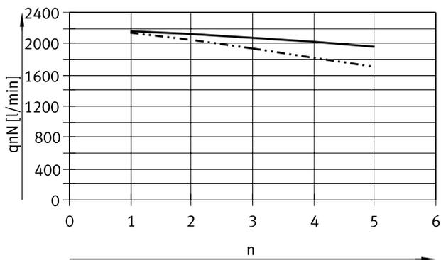
— Standard nominal flow rate per valve on standard manifold rail
