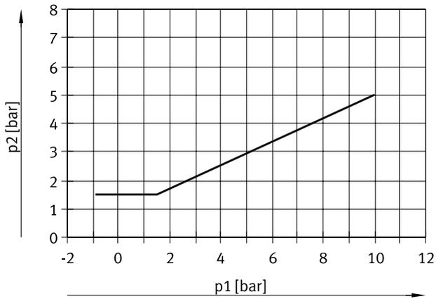
**Size 25 – Pilot pressure p2 as a function of working pressure p1**
