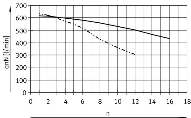
— Standard nominal flow rate per valve on standard manifold rail
