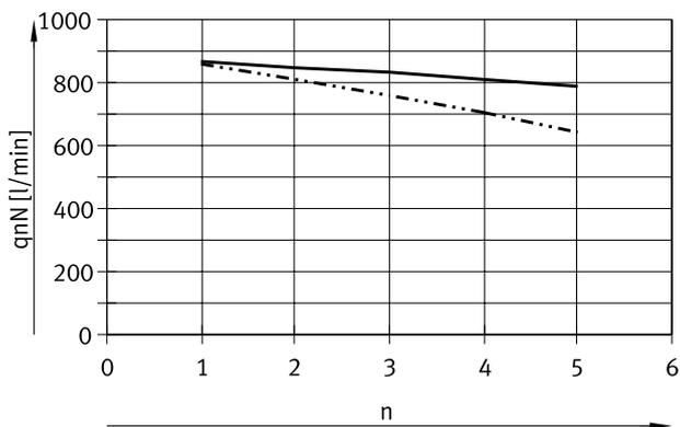
— Standard nominal flow rate per valve on standard manifold rail
