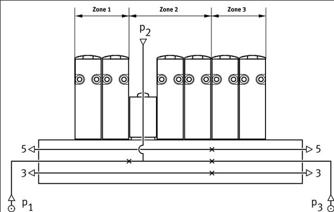
The number of pressure zones with the VTUS is limited by the number of valve positions on the manifold block/common supply manifold. Note that each supply plate occupies one valve position. There must always be at least 2 valve positions between 2 separators. In the case of a maximum extension of 16 valve positions, a maximum of 9 pressure zones can be created.
