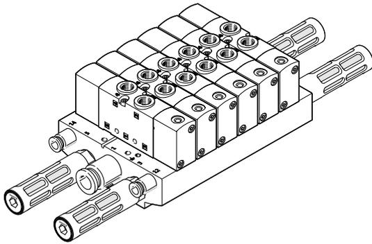
In-line valves are designed to be used without being linked pneumatically. All pneumatic connections are on the valve and can be equipped with fittings/tubing. By using a special seal set, the in-line valves can also be mounted on a manifold rail (pneumatic linking) as semi in-line valves.
