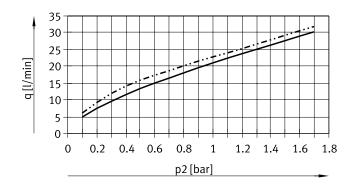
Flow plotted against voltage at room temperature, operating pressure 1.7 bar
