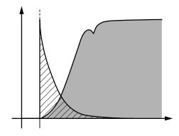
Compared with solenoid valves, proportional valves with piezo technology require virtually no energy to maintain an active state thanks to their capacitive principle. The piezo valve operates like a capacitor: it needs current only at the start in order to charge the piezoceramics.
