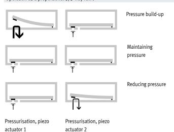
The piezo actuators installed in the valve VEMP proportionally regulate both the pressure and flow rate for pressurisation and ensure proportional exhausting.
