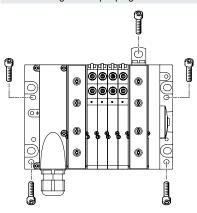
The MPA-L valve terminal is screwed onto the mounting surface using four M4 or M6 screws. The mounting holes are on the multi-pin plug connection and on the right-hand end plate.
