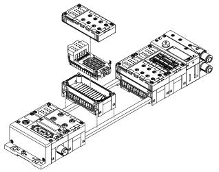
The mechanical connection between the CPX modules is established using tie rods. Two screws in the end plates are all that are needed to assemble the entire unit.
