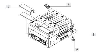
A holder VMPAL-ST-AP-10 (part no. 561109) with inscription labels (part no. 18576, IBS-6x10) can be mounted on each sub-base for labelling the valves.
