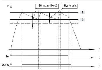
If the desired threshold value [1] for the vacuum is reached, vacuum generation is automatically switched off. A check valve prevents a decrease of the vacuum. Nonetheless, leakage (e.g. due to rough workpiece surfaces) will slowly reduce the vacuum. If the vacuum drops below the threshold value [2], vacuum generation is automatically switched on. Vacuum is generated until the set threshold value [1] is reached again.
