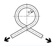
The tube is bent in the direction of its own curve until the tubing outer diameter is flattened by 5%.
