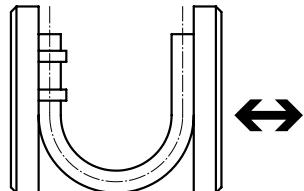
The tube fixed to the base plate is bent until the deformation results in a kink. The measured value is the minimum bending radius Rmin. This Rmin results in significant reductions in the flow rate.
