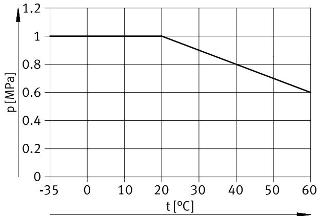
**Operating pressure p as a function of temperature t (medium: water)**
