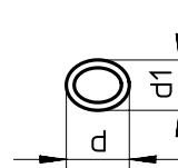
Cross-section flattened by bending the tube.
