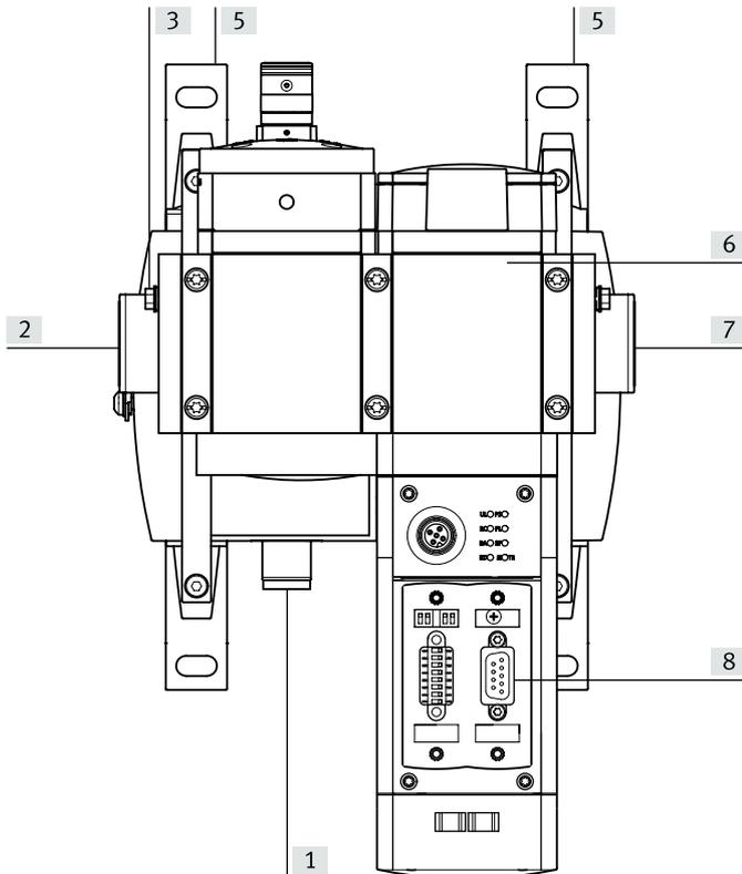
The MSE6-E2M consists of the following main components: shut-off valve, flow sensor, pressure sensor and bus node. The fieldbus interface enables it to be connected to a higher-order controller, e.g. a system or machine controller.
