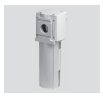
Active carbon filters remove liquid and gaseous oil particles as well as odor and taste from compressed air. Pre-filtration with a grade of 0.01 micron is required.
