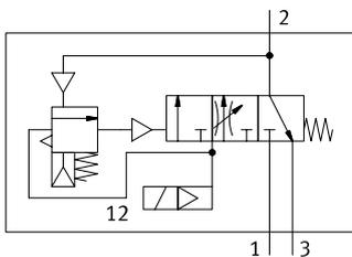
Electropneumatic soft-start/quick exhaust valve for gradual pressurisation and quick exhausting of system components (single channel).
