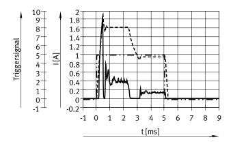
Current in the supply line at 24 VTrigger signalCoil current
