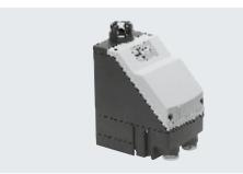
Condensate passes through the connecting bore in the bottom of the filter bowl into the attached condensate drain valve, where it is collected in a reservoir. A capacitive sensor detects when the maximum filling level is reached.
