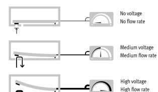
The piezo actuators are actuated using variable voltage to give proportional control.
