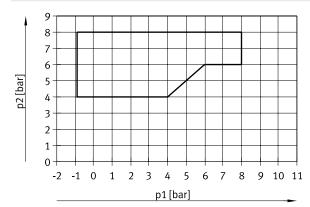
For valves in width 20 mm with code for position function 1-32: MS, NS, KS, HS, DS  $\,$
