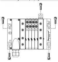
The MPA-L valve terminal is screwed onto the mounting surface using four M4 or M6 screws. The mounting holes are on the multi-pin plug connection and on the right-hand end plate.
