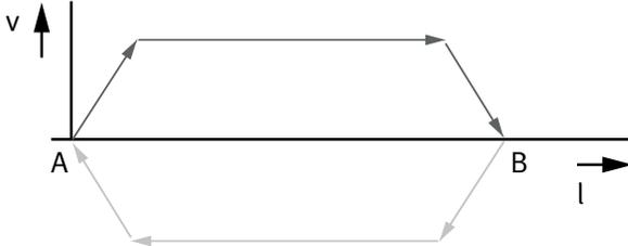
Extended motion profile for simplified press-fitting and clamping functions: with speed and force control
