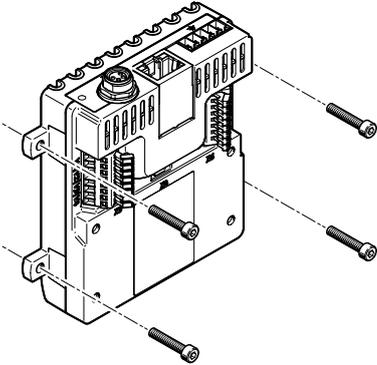
Sturdy wall mounting of the valve control module using four through-holes.
