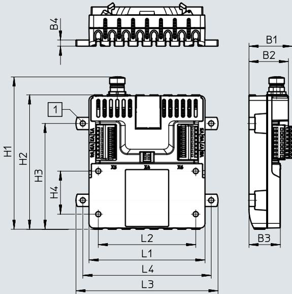
[1] Mounting holes  $\varnothing 3.4$  for M3 socket head screw
