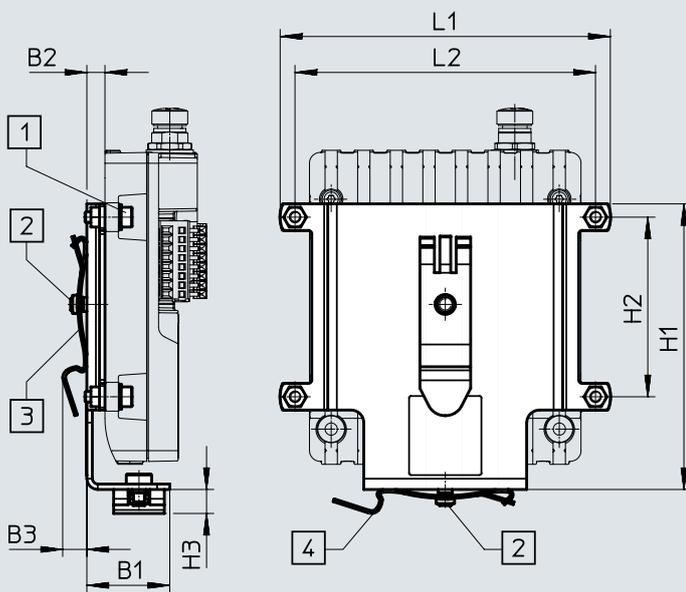
[1]  $\varnothing 3.2$  for M3 socket head screw
