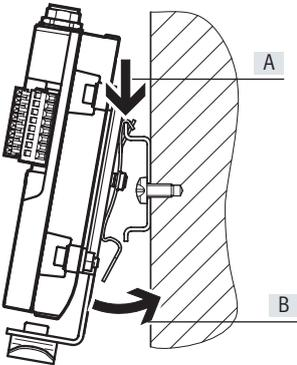
The H-rail mounting VAME-V3-H consists of a mounting bracket and a clamp:
