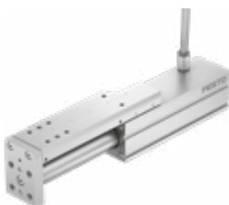
Air is exchanged between the interior of the cylinder and the environment via a sealing air connection. This prevents negative pressure or excess pressure arising in the interior of the cylinder.
