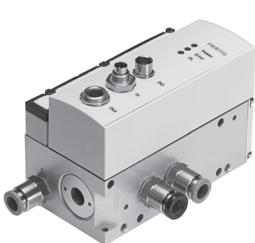
The 5/3-way proportional directional control valve for applications with Soft Stop and pneumatic positioning. Fully digitalised – with integrated pressure sensors, with new diagnostic functions. In sizes 4, 6 and 8. Flow rate of 350, 700 and 1400 l/min.
