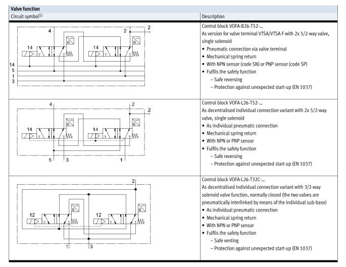
1) The symbol represents a valve with a proximity sensor with a switching output signal, in the illustration an N/O contact. In accordance with ISO 1219-1, this symbol applies to both N/O contacts and N/C contacts. The switching element function of all sensors used here is an N/C contact.
