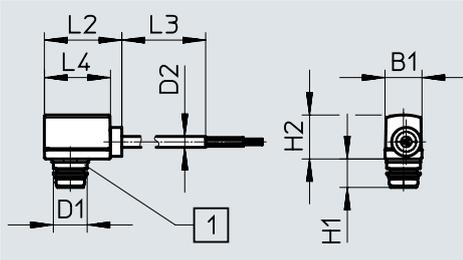
[1] Supply port: pin-type cartridge
