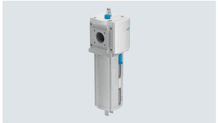
The proportional lubricator adds a precisely adjustable amount of oil to the compressed air. The pressure drop that occurs when air flows through a Venturi nozzle is used to feed oil from the container to the drip cap.
