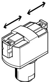
The indicated opening and closing times [ms] have been measured at room temperature and 6 bar operating pressure with vertically mounted gripper and without external gripper fingers. Load is increased if external gripper fingers are attached. This means that kinetic energy is also
