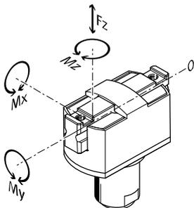
The indicated permissible forces and torques apply to a single gripper jaw. The indicated values include the lever arm, additional applied loads caused
