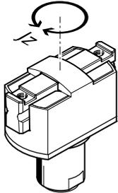
Mass moment of inertia [kgm<sup>2</sup>x10<sup>-4</sup>] for parallel grippers in relation to the central axis, without external gripper fingers, without load.
