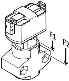
Theoretical actuating force due to stroke compensation for design variant with stroke compensation.
