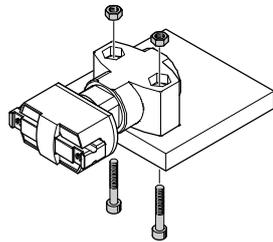
With flange mounting, screws and dowel pins
