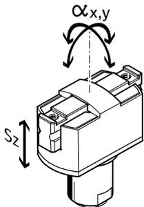
With parallel grippers, backlash occurs between the gripper jaws and the guide element due to the plain-bearing guide. The backlash values listed in the table have been
