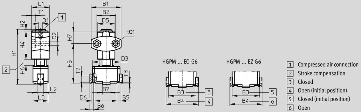
With clamping spigot – HGPM-...-E...-G8
