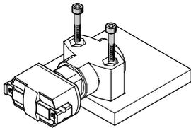
With through-holes, screws and retaining nuts
