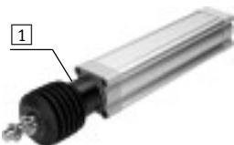
The protective bellows kit is a leak-free system. To prevent unwanted media from being drawn in, the supply and exhaust air for the kit must be ducted via a pressure compensation hole in the connection part [1].
