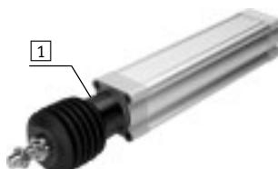
The protective bellows kit is a leak-free system. To prevent unwanted media from being drawn in, the supply and exhaust air for the kit must be ducted via a pressure compensation hole in the connection part [1]. The kit protects the piston rod, seal
