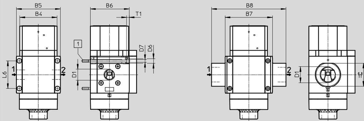
1 Mounting screw M6x11.90 to DIN 912 (not included in the scope of delivery) for wall mounting without mounting bracket
