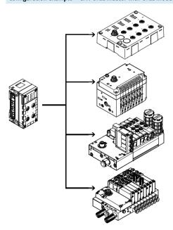
The CPX-CTEL master provides 4 external I-Port interfaces, to each of which a device can be connected. I-Port is an interface for the exchanging of serial data for connecting decentralised modules or valve terminals from Festo. The I-Port interface is based on IO-Link and is compatible with it in certain areas. The connection type corresponds to a star topology. In other words, only one module or valve terminal can be connected to each I-Port.
