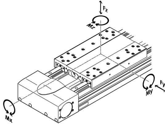
If the axis is subjected to more than two of the indicated forces and torques at the same time, the following equation must be satisfied in addition to the indicated maximum loads:
