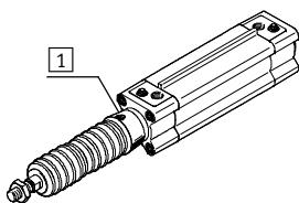
The bellows kit is a leak-free system. To prevent unwanted media from being drawn in, the supply and exhaust air must be ducted via a pressure compensation hole in the connection part 1.
