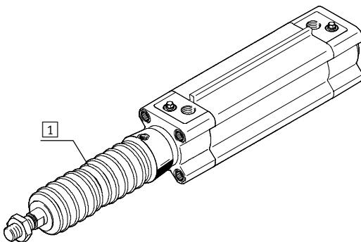
The protective bellows kit is a leak-free system. To prevent unwanted media from being drawn in, the supply and exhaust air must be ducted via a pressure compensation hole in the connection part 1. The kit protects the piston rod, seal
