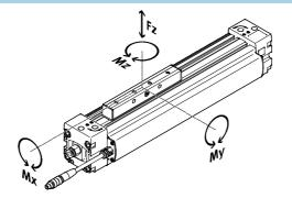
If the drive is simultaneously subjected to several of the forces and torques listed below, the following equation must be satisfied in addition to the indicated maximum loads:
