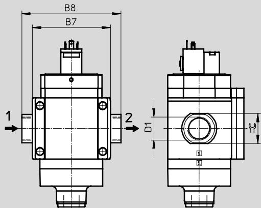
[1] Mounting screw M6xmin.90 to DIN 912 (not included in the scope of delivery) for wall mounting without mounting bracket
