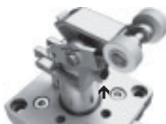
Sensing of the toggle lever position
