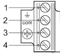
Pin allocation if cables are connected by the customer
