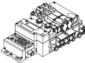
An integrated fieldbus node manages the communication connection to a higher-order PLC. This enables a space-saving pneumatic and electronic solution.
