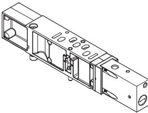
With this plate a valve can be shut off from the supply pressure of the terminal. This means that the valve can be removed without shutting off the pressure.
