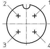
Pin allocation M12 on individual valve to ISO 20401
