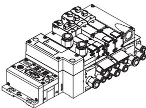
Controllers integrated in the Festo valve terminals permit the construction of stand-alone control units to IP65, without control cabinets.
