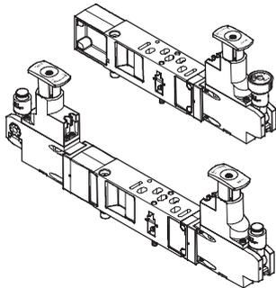
An adjustable pressure regulator can be installed between the sub-base and the valve in order to control the force of the respective actuator.
