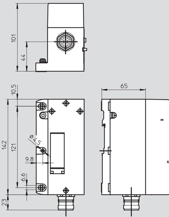
**Valve terminal type 44 VTSA, type 45 VTSA-F optimised flow**
