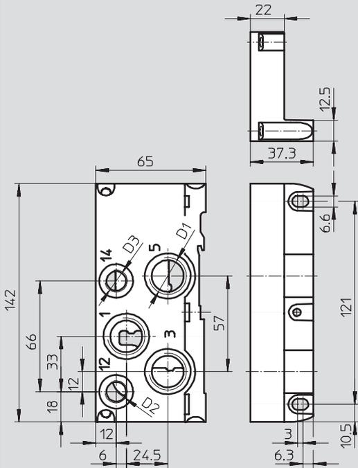
Right-hand end plate with coding cap
