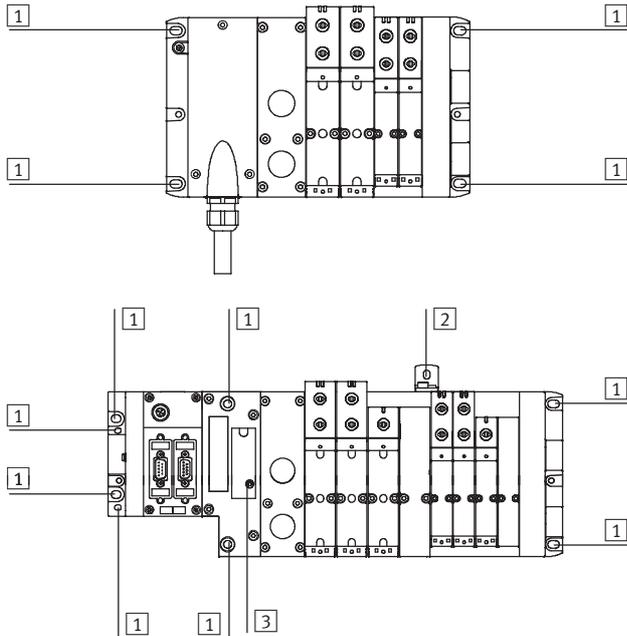
The VTSA/VTSA-F valve terminal is screwed onto the mounting surface using M6 screws. The mounting holes are located at the following points:
