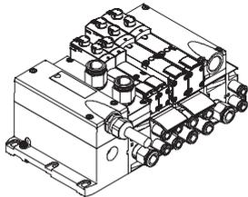
Control signals from the controller to the valve terminal are transmitted via a pre-assembled multi-wire cable or a self-assembled multi-pin plug connection (Cage Clamp), which substantially reduces installation time.
