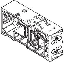
VTSA/VTSA-F is based on a modular system which consists of manifold sub-bases and valves. Manifold sub-bases are available for valve width 18 mm and width 26 mm in a double grid, i.e. two valves per manifold sub-base. The manifold sub-base contains a ducting seal and electrical linking. They can be freely mixed within a
