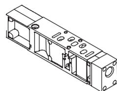
With this plate a valve can be supplied with individual operating pressure independently of the operating pressure of the terminal.
