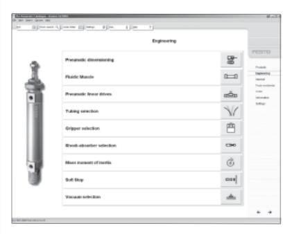
No matter whether discs, blocks, push-on flanges, grippers, etc: This tool does the job of calculating all mass moments of inertia for you. Just save, send, or print - and you're finished.
