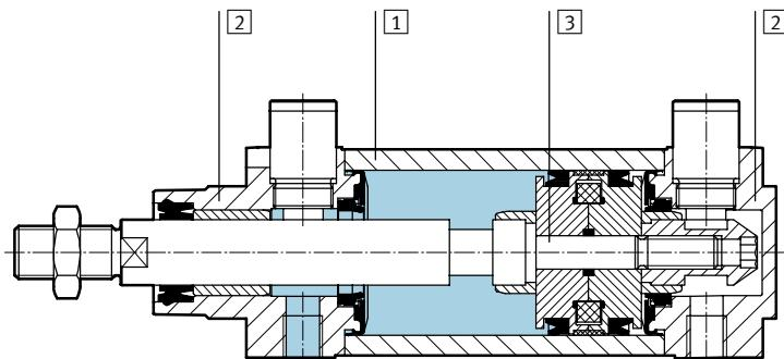
Cylinder with clamping cartridge
