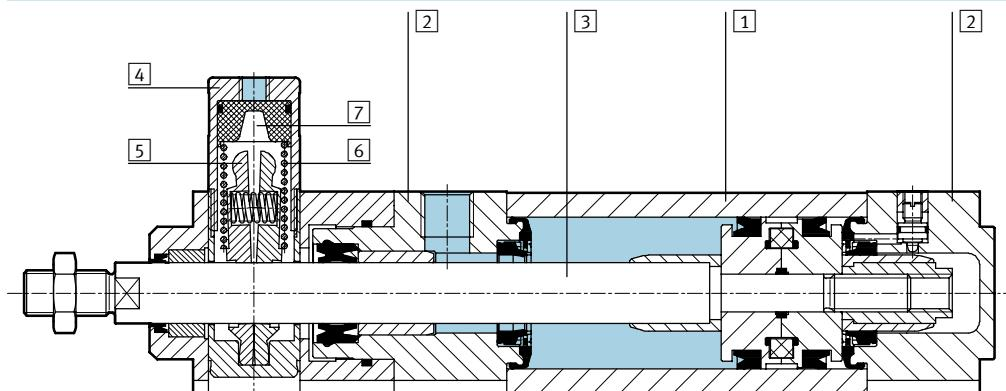
Cylinder with clamping cartridge
