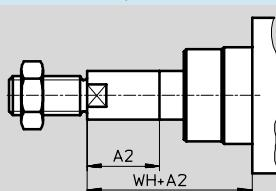
In combination with variant S2, the piston rod is extended on one side at the bearing cap. The clamping unit is
