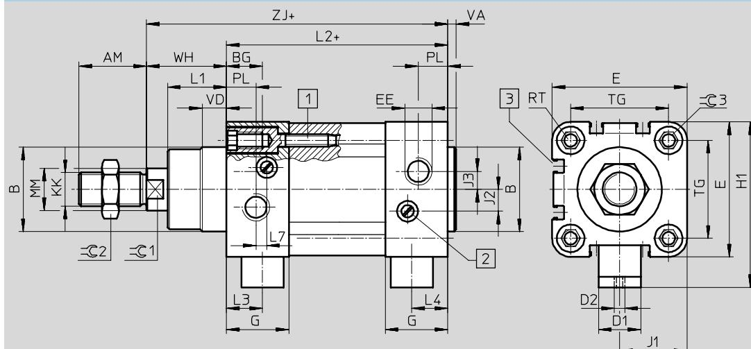
[1] Socket head screw with female thread for mounting attachments
