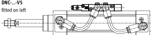
Double solenoid valve unactuated, piston rod retracted
