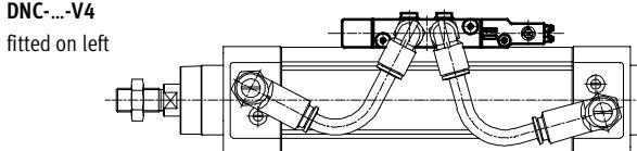
Single solenoid valve unactuated, piston rod advanced
