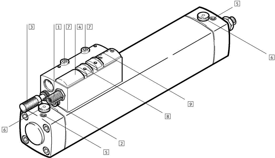
1 Multi-pin connection, M12 plug, 8-pin
