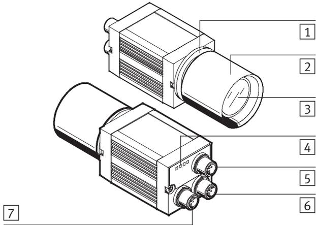
Fig. 1/4: Display and connecting elements in SBOC-Q
