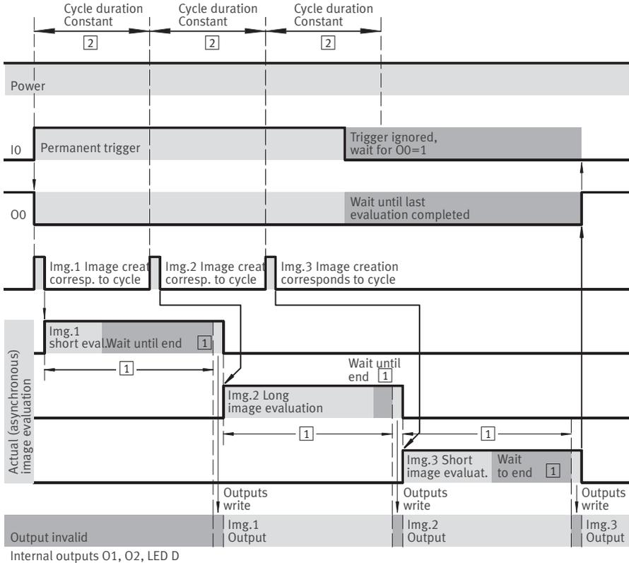
Fig. 4/13: “Fixed frame rate” evaluation mode – signal curve using system parameters
