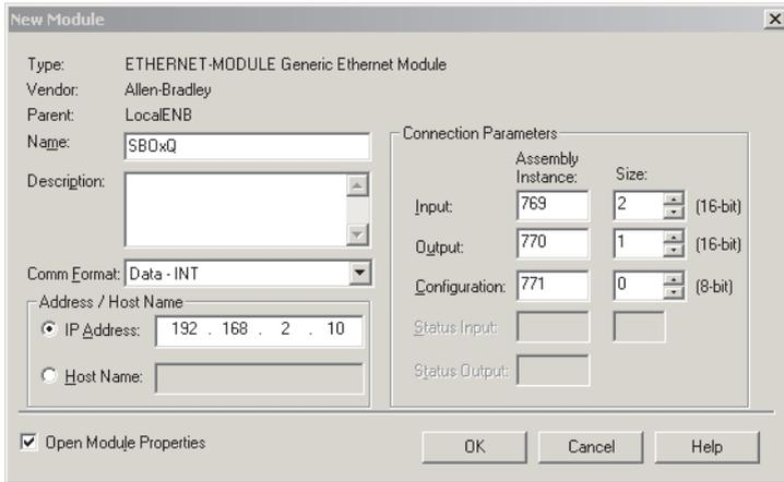
Fig. 4/30: Configuration of the EtherNet/IP module
