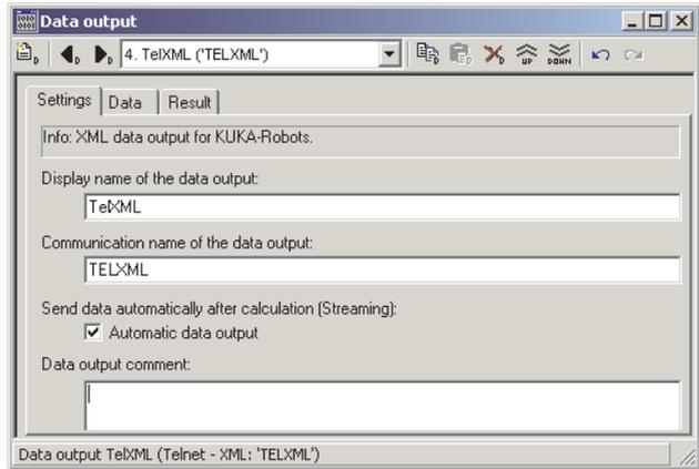
Fig. 4/22: Configuring data output with Telnet streaming
