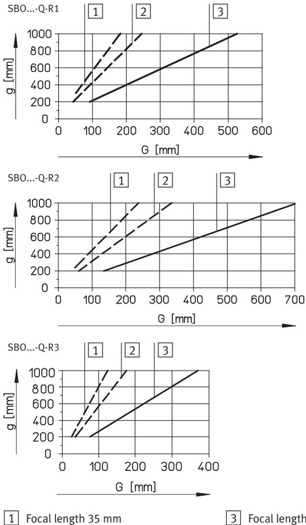
Fig. 1/5: Working distances  $g$  [mm] and object size  $G$  [mm] for typical fixed focal lengths
