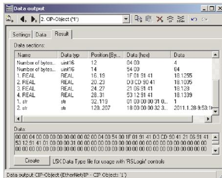
Fig. 4/31: Data output of the EtherNet/IP module
