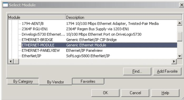
Fig. 4/29: Selecting the Ethernet module
