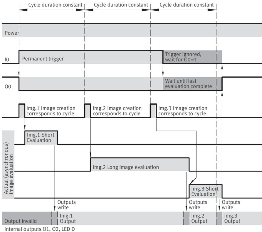
Fig. 4/12: “Fixed frame rate” evaluation mode – signal curve with standard settings
