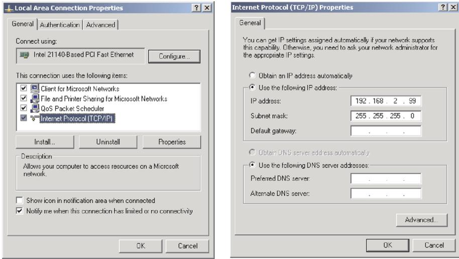
Fig. 4/2: Characteristics of LAN connections and characteristics of Internet Protocol (TCP/IP)
