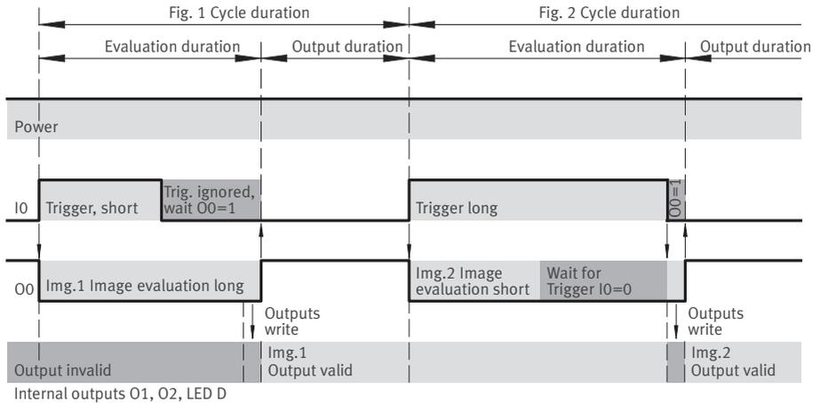
Fig. 4/5: “Triggered” evaluation mode – Signal curve with standard settings
