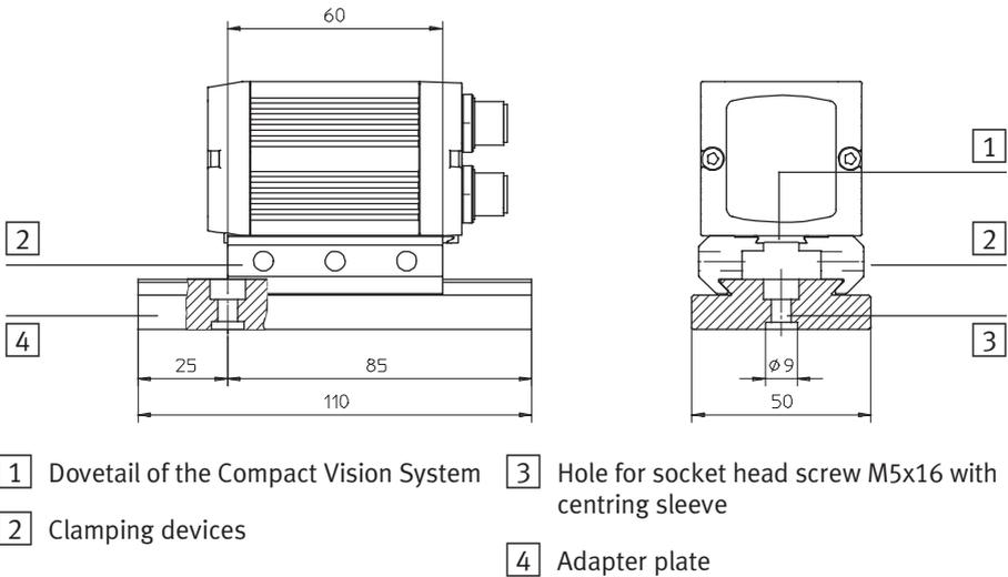
Fig. 2/3: Mounting with adapter kit type SBOA-HMSV-39
