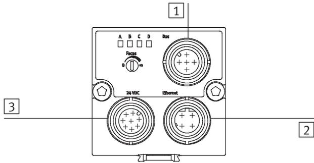
Fig. 3/1: Electrical connections of the SBO Compact Vision System
