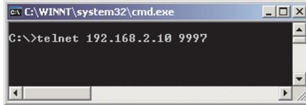
Fig. 4/23: Starting the Telnet program via the command line
