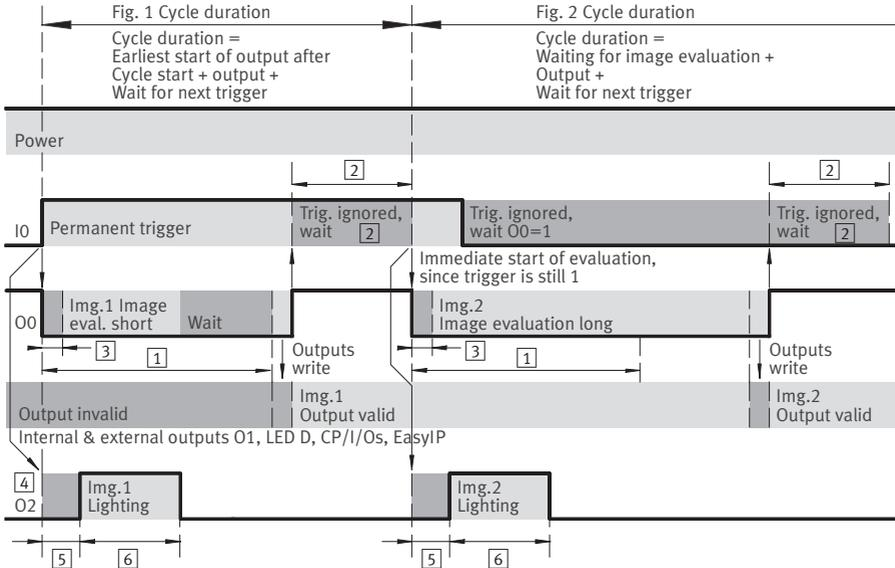
Fig. 4/9: “Free run” evaluation mode – Signal sequence using system parameters
