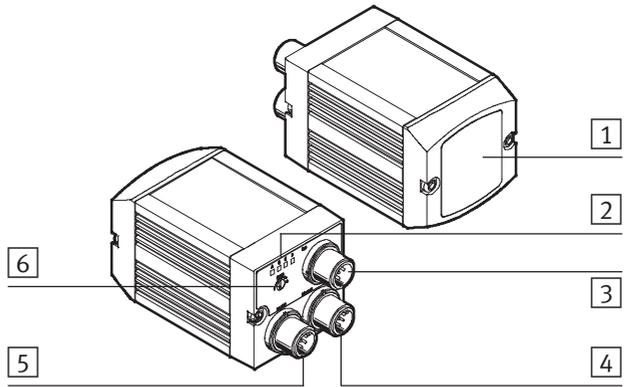
Fig. 1/3: Display and connecting elements in SBOI-Q
