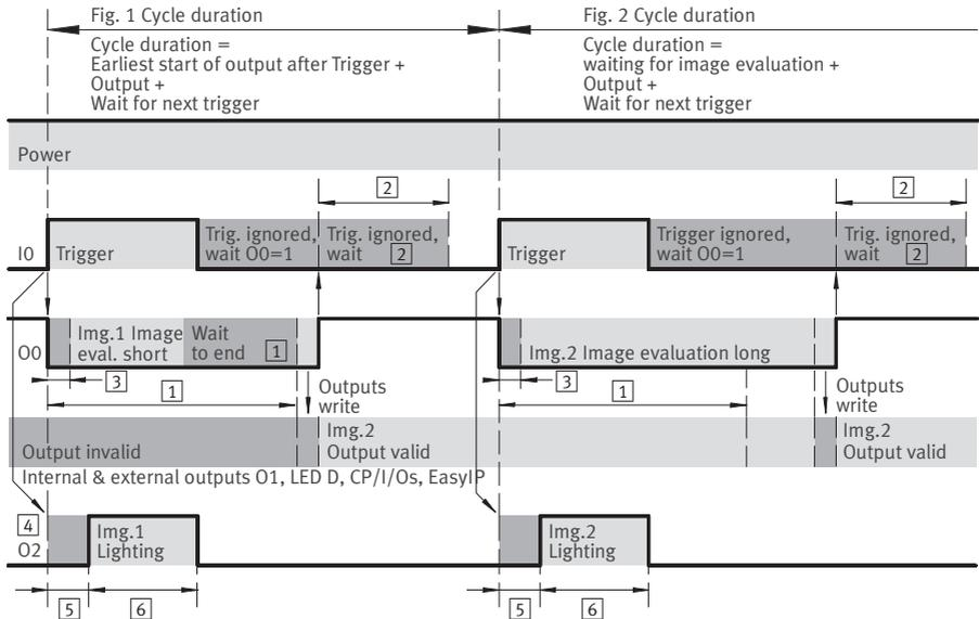
Fig. 4/7: “Triggerred” evaluation mode – Signal sequence using system parameters – Case 2
