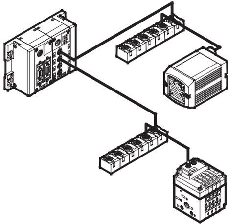
Fig. 4/16: Example line assignment: Compact Vision System SB01-Q as CPI module
