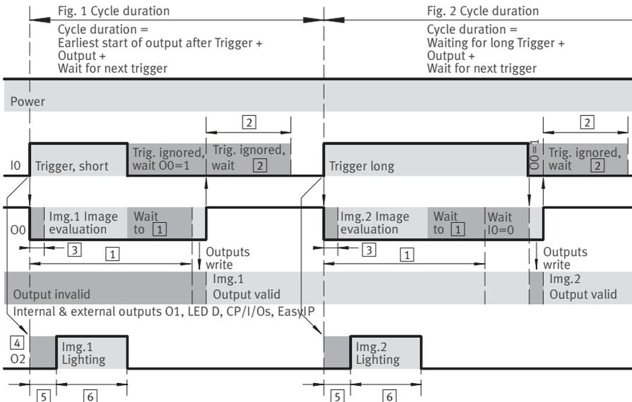
Fig. 4/6: “Triggered” evaluation mode – Signal sequence using system parameters – Case 1
