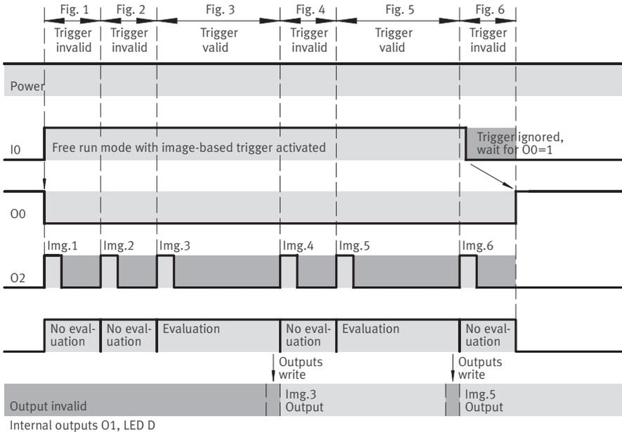
Fig. 4/11: Free run mode with image-based trigger
