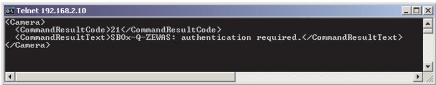
Fig. 4/24: Telnet program with SBO...-Q acknowledgement (here with authentication)
