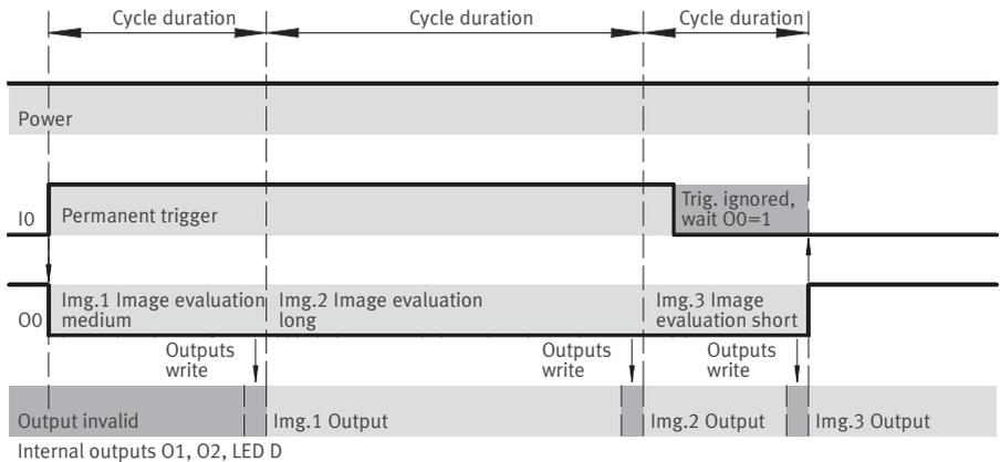
Fig. 4/8: “Free run” evaluation mode – Signal sequence with standard settings
