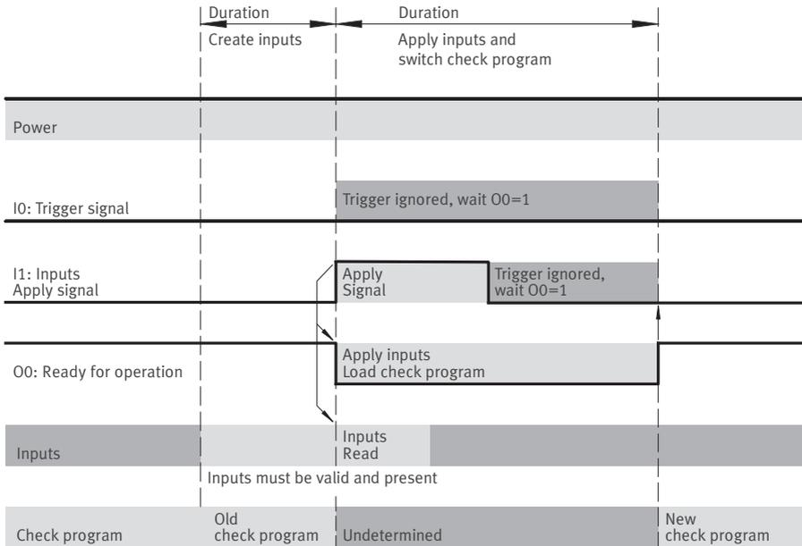
Fig. 4/14: Signal curve: Apply inputs – Switch check program
