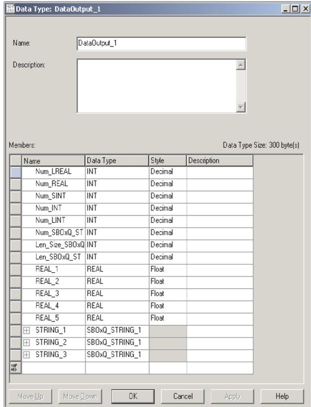
Fig. 4/34: Structure of an imported data type
