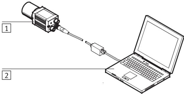
Fig. 1/1: Direct networking with the PC
