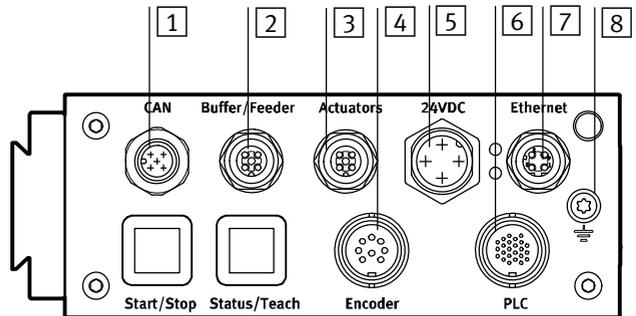
Fig. 2/4: Connections of the Checkbox
