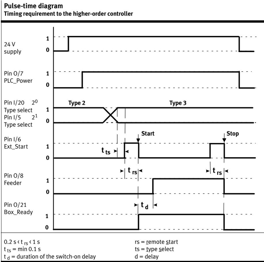
Tab. 3/11: Pulse-time diagram: Timing requirement to the higher-order controller
