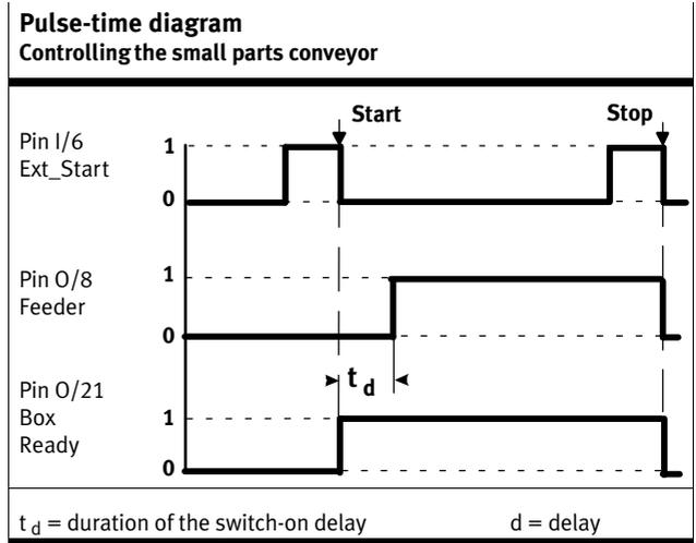
Tab. 3/20: Pulse-time diagram: Control of the small parts conveyor
