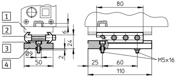
Fig. 2/2: Mounting the Checkbox with connecting kit HMSV-12
