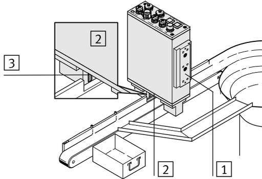
Fig. 2/3: Arrangement of the Checkbox over the transporting device (example)
