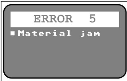
Fig. 2/9: Example: Error message “Error 5”
