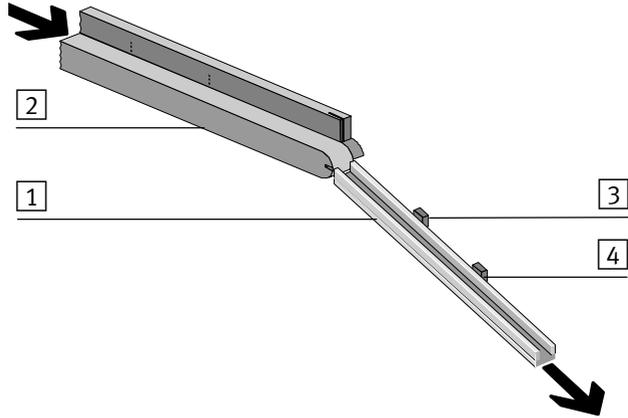
Fig. 3/7: Buffer zone check with switching delay
