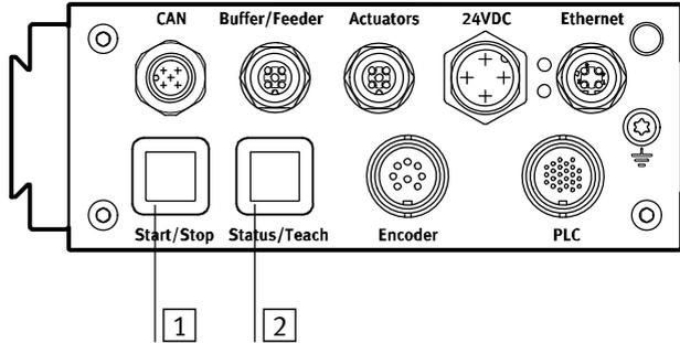
Fig. 2/5: Display and control elements
