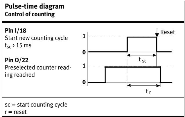
Tab. 3/17: Pulse-time diagram: Control of the counting procedure
