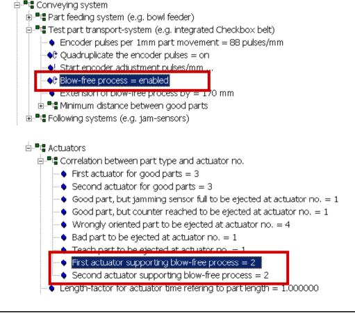
The rejection process can be aktivated and deactivated with the parameter described on the left.
