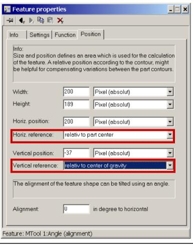
Both the horizontal and the vertical relation to the placement of tools additionally defined in CheckOpti (e. g. ROI) can be, in operating system 3.2,
