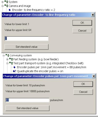
With operating system 3.2 the parameter "Encoder- to line-frequency ratio" allows values of up to 64.
