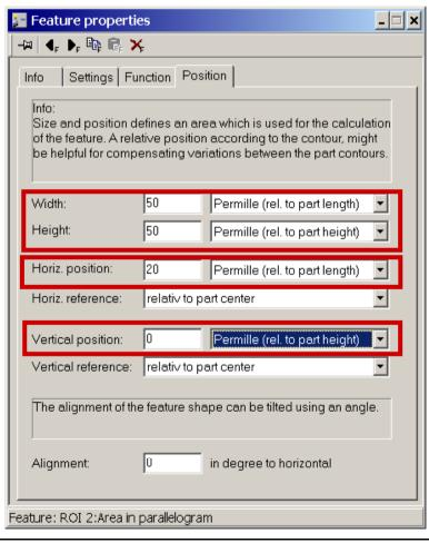
The size and position of the tools that can be additionally defined in CheckOpti
