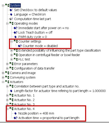
If the counter mode of Checkbox Compact is **deactivated**, four actuators for the assignment to parts categories (good part, bad part, etc.) are available.
