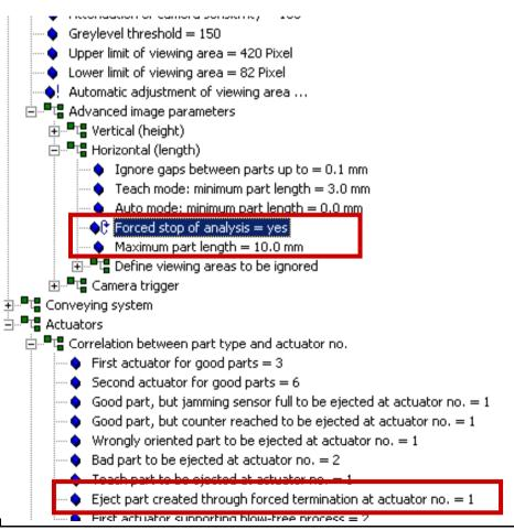
If the function "Forced termination of analysis" responds because a test part is too long, OS3.2 allows to assign a separate actuator output to the parts thus generated.
