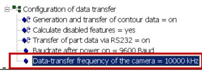
Change of parameter: Data-transfer frequency of the camera
