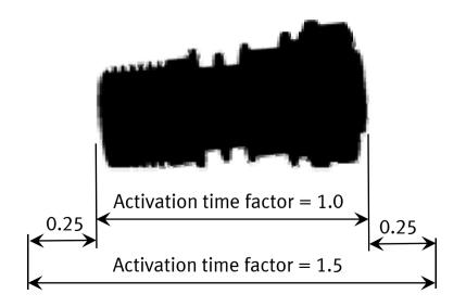
"Proportional to part length", the relevant actuator is triggered for the time defined in "Length of the part/belt speed".
