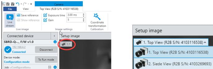
Remark: The numbering of the camera is independent from the USB connector on the device! It is only a definition in the software! The assignment is based on the serial-no. of the camera device. If camera has to be exchanged you have to assign the new device in Set-up, otherwise you get an Error: "Camera type match failed"
