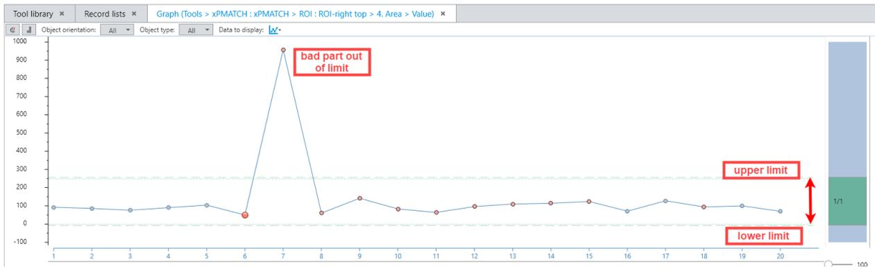
To change the value for the display, you can select another feature in the Tool structure or in any other window. Or do a selection in the “Data to display” drop down menu.
