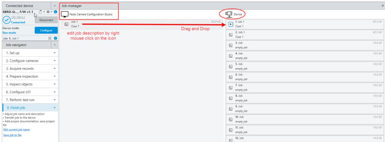
By drag on the job on left side and drop it on a memory on right side, the setting are stored on the device. The “play” button show the selected job which is processed in run mode.
