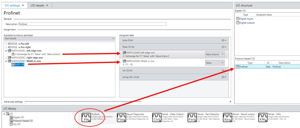
In principle the same procedure as in use case 1. Assign the data by drag and drop.
