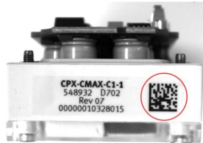
The red marked area must be inspected. It has to be checked whether all 4 screw at the corner of the module are mounted and if only 4 of the maximum of 8 LED are available.(count LED)
