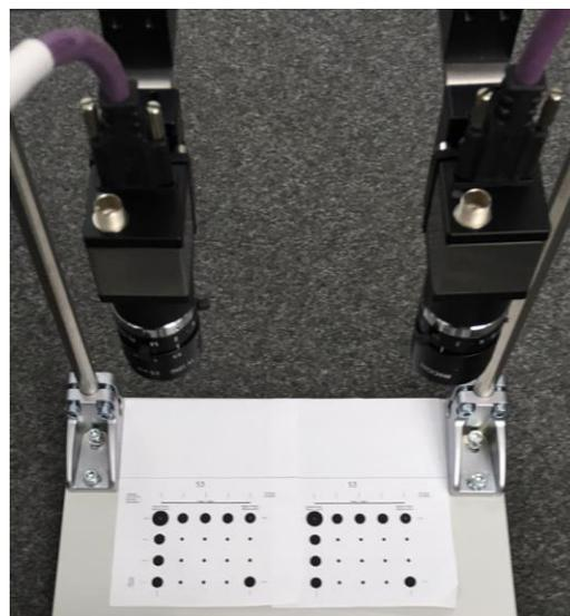
If the field of view is determined, you can print the calibration pattern, that it fits to that size. It should not be smaller than 80% of this area.
