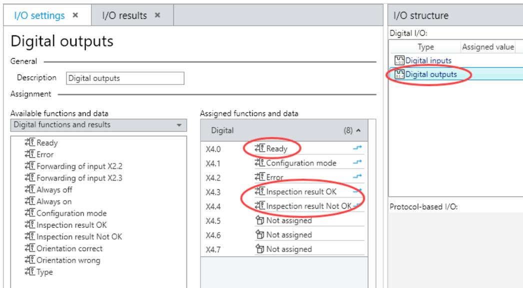
To use the result of the 2D code, we need to set up a dataoutput for the communication to a PLC controller.
