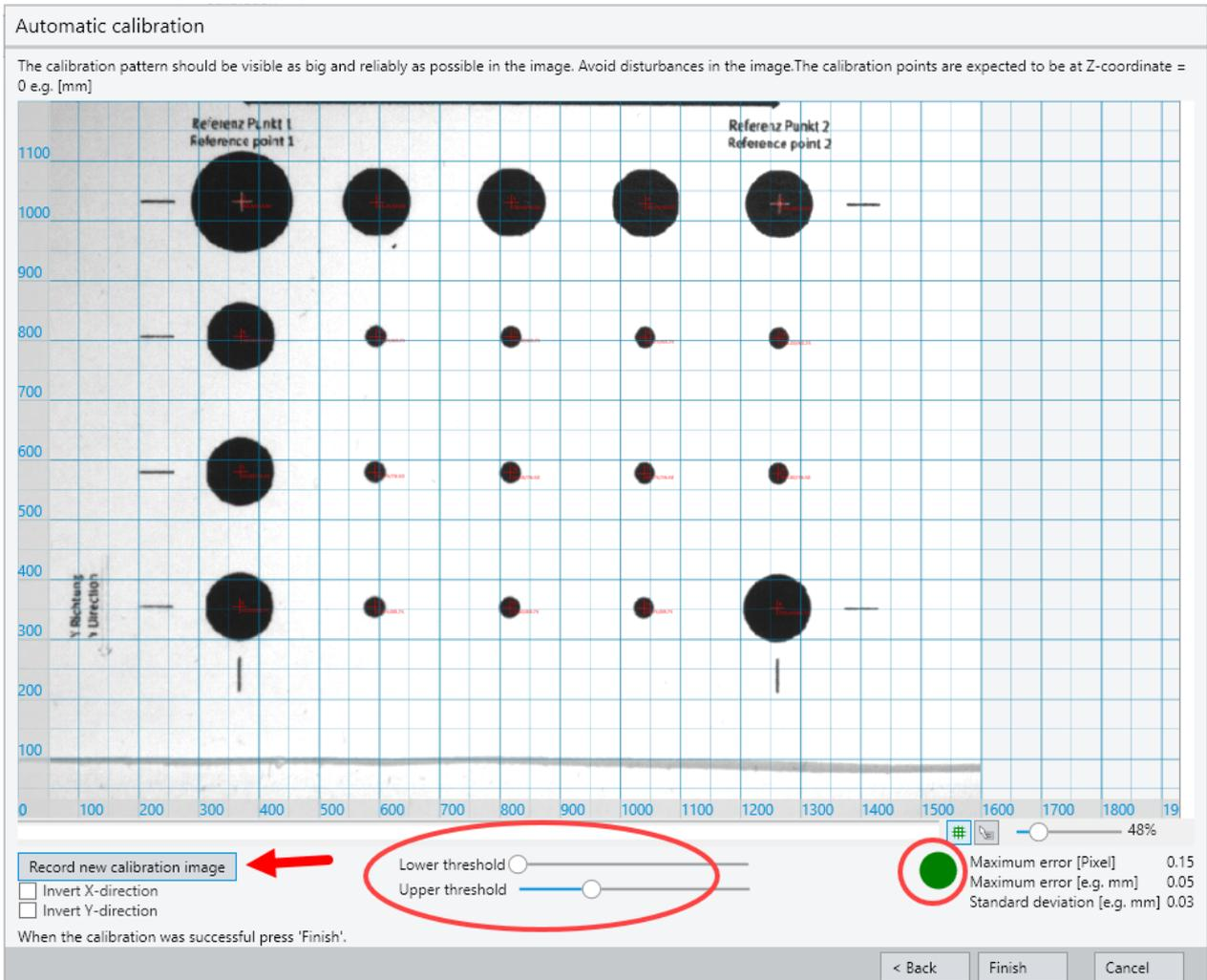
Press the “Record new calibration pattern image”-button. Then an image is captured and evaluated. If the green dot appear, the calibration was successful. If the dot is red: Try different setting of the threshold sliders to achieve a better image until the dot get green.
