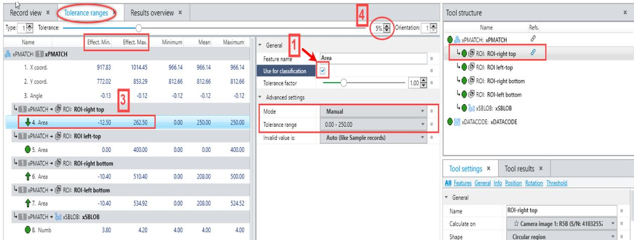
Every “used for classification” feature has to be within the limits, which is displayed in the column Effect. Min and Effect. Max. values.(3) This limits are calculated on the general tolerance(4): Default 5%
