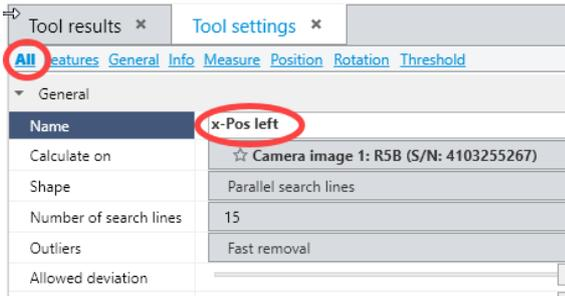
Now we can copy and paste the tool in Tool structure for the right edge of the band.
