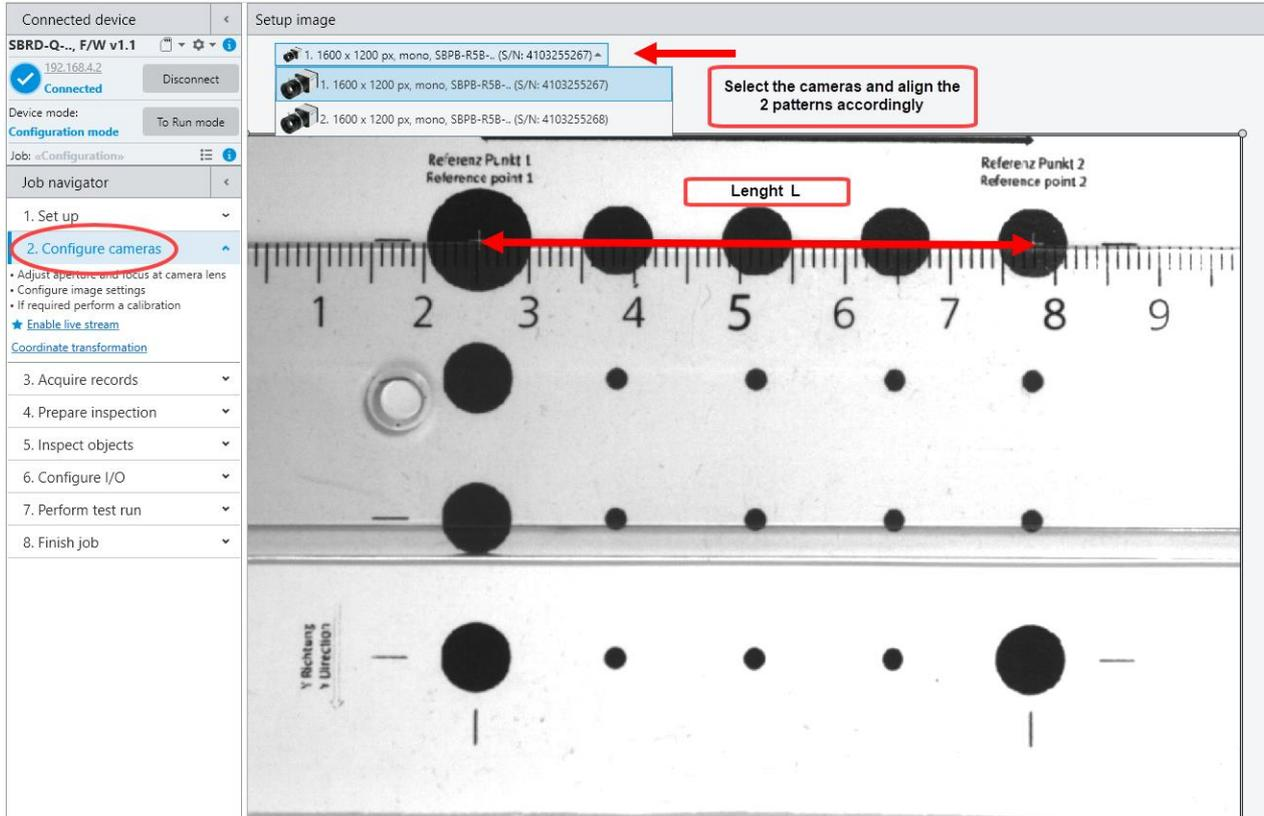
It is not possible to have a view of both cameras simultaneously! So in this example, a ruler help for the alignment process!
