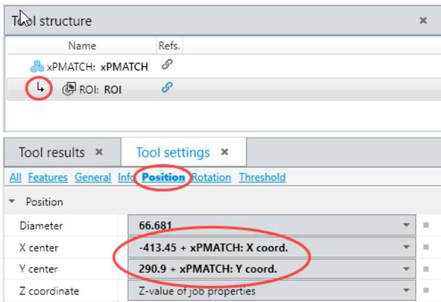
In the tool settings tab Position you can see the reference and the offset for the ROI. As well in the tab Rotation the xPmatch references are connected.
