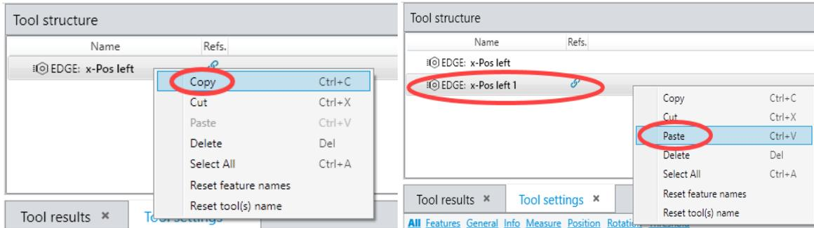
The copied tool has to be adjusted for the right side. There we select the second camera, adapt the tool name and the search direction of the edge detection:
