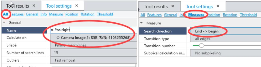
In the image we should see the tool now on the right side of the band. And the search lines starting from right side.
