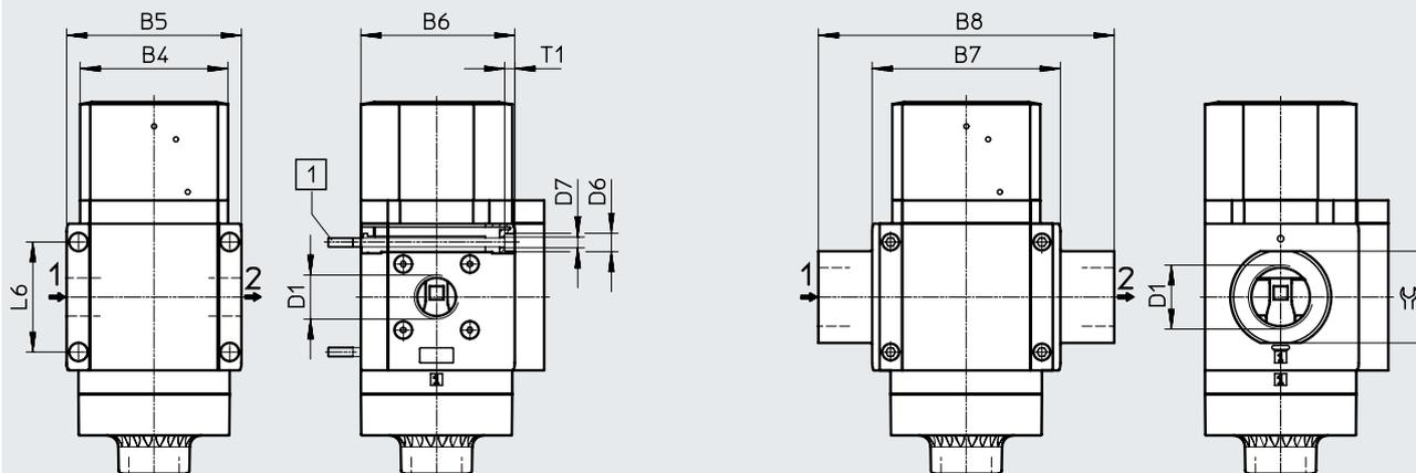
[1] Retaining screw M6xmin. 90 to DIN 912 (not included in the scope of delivery) for wall mounting without mounting bracket
