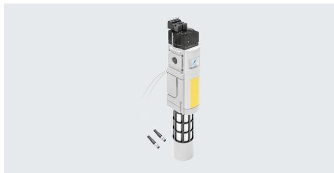
The electropneumatic soft-start/quick exhaust valve is used to reduce pressure quickly and safely and to build up pressure gradually in industrial pneumatic piping systems and terminal equipment.
