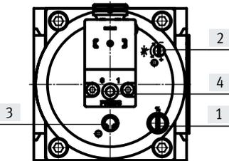
[1] Screw for adjusting the pressure switchover point
