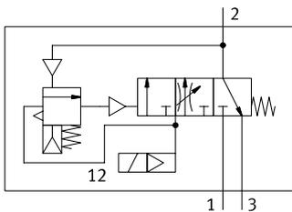
Electropneumatic soft-start/quick exhaust valve for gradual pressurisation and quick exhaust of system components (single channel). The main restrictor in the cover permits a slow build-up of the output pressure p2. Once the output pressure p2 has reached the set pressure switchover point (switching pressure), the valve opens and the full operating pressure p1 is available at the output
