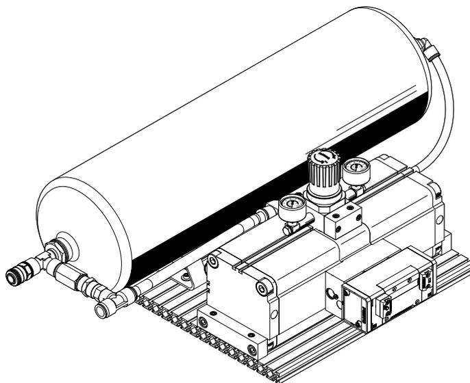
Combination of pressure booster, air reservoir in stainless steel, bypass with check valve for constant filling of the air reservoir with the system pressure, pressure gauge set, silencer, fitting and quick coupling. Combination completely mounted on a profile plate.
