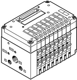
Control signals from the controller to the valve terminal are transmitted via a pre-assembled multi-core cable, which substantially reduces installation time. The current reduction for the valves is also integrated in the multi-pin plug connection.
