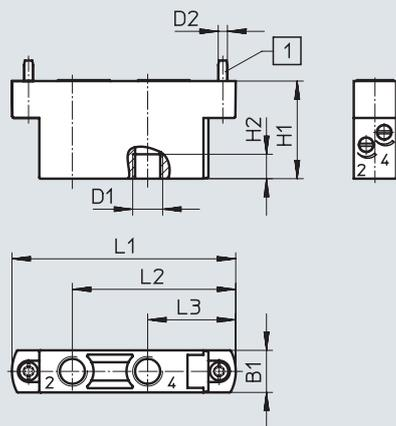
[1] Retaining screw enclosed separately
