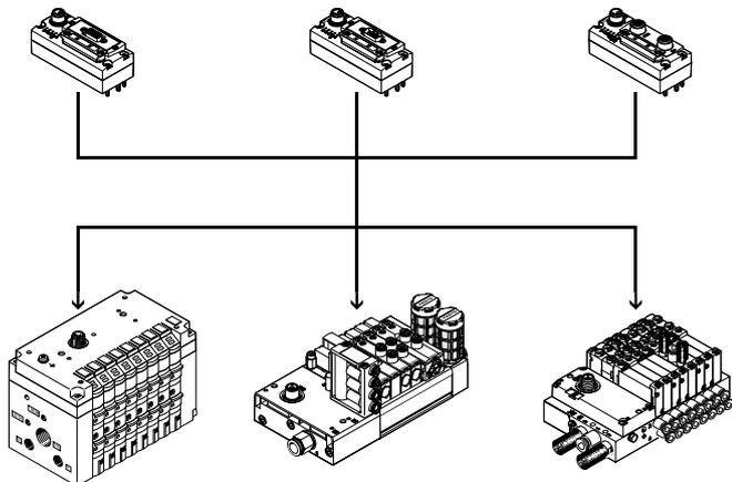
CTEU is a system for the compact connection of a valve terminal to different fieldbus standards such as PROFIBUS and DeviceNet®.
