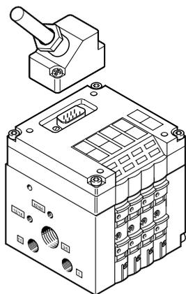
The multi-pin plug connection provides electrical integration in addition to pneumatic integration and enables the control cabinet and the valve terminal to be connected using a single cable.
