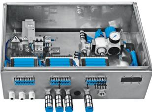
Using a pneumatic multiple connector plate (code GQC, GQD, GQE), valve terminals CPV can be installed directly in the housing wall with a suitable opening. This ensures tubing connections are on the outside of the control cabinet.
