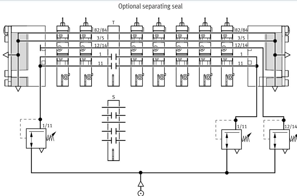
Internal pilot air supply, ducted exhaust air or threaded silencer
