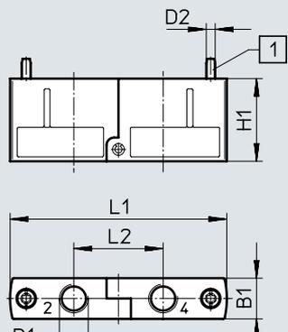
[1] Retaining screw enclosed separately
