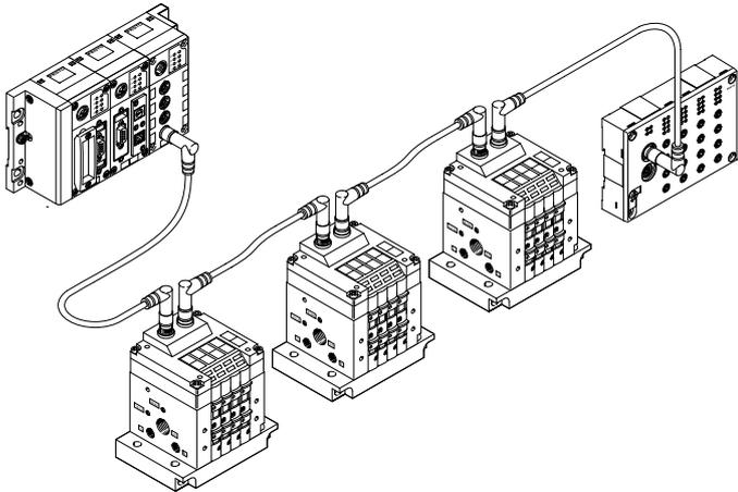
The installation system CP/CPI comprises an interface for connecting valve terminals and I/O modules with CP connection to the modular electrical terminal CPX.
