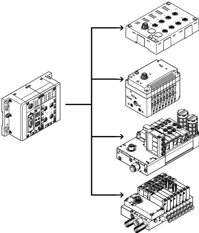
A CTEL system consists of the CTEL master and the devices with I-Port interface, which are connected using special connecting cables. This permits a decentralised layout of the devices. This means that the valve terminals and I/O modules with I-Port interface (devices) can be mounted very close to the cylinders to be controlled. This reduces the length of the air supply lines used, which in turn minimises flow losses as well as pressurisation and exhaust times.
