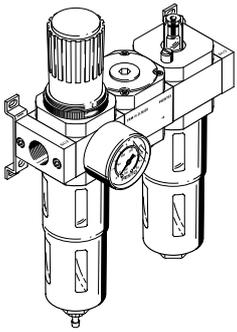
[KB] Filter regulator, branching module with pressure switch and lubricator
